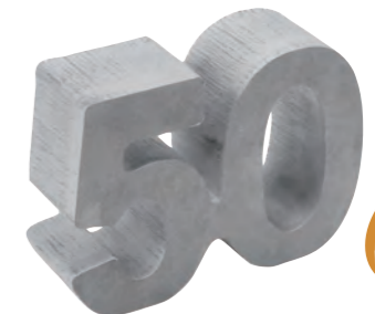
Material: Aluminum Thickness: 50mm Assist Gas: Nitrogen
