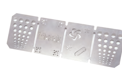
Material: Mild Steel Thickness: 1.0mm Assist Gas: Nitrogen
