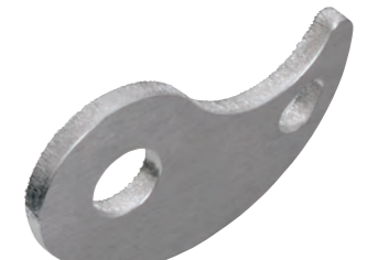
Material: Aluminum Thickness: 5.0mm Assist Gas: Nitrogen
